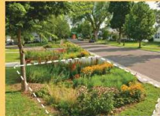
Fig. 2.53 Reference images of Raingarden (Buildings)
