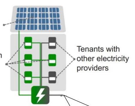
Surplus electricity is feeded in, missing electricity is drawn from the grid
