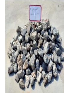
Aggregate +- 20 to 40 MM
