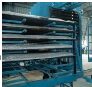
Board preparation by hot and cold press
